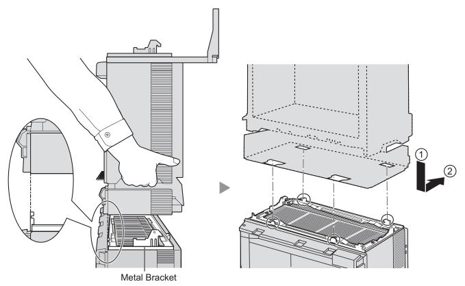
**5.** Secure Expansion Shelf 1 to the metal bracket with 2 screws (B).
