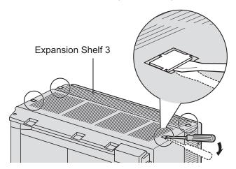
**4.** Fasten the wall brackets loosely to Expansion Shelf 3 with 4 screws (D). (This makes it easy to adjust the position of the shelves later.)
