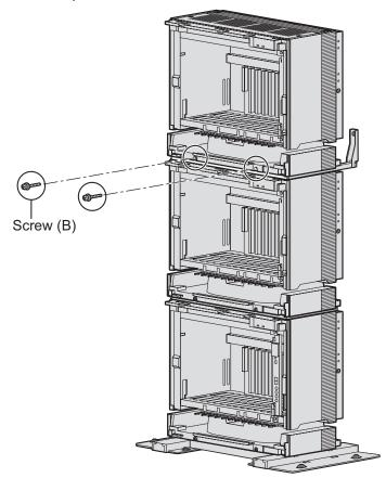
Installation of a 3-shelf system is complete. Next, it is necessary to connect the shelves. If you are installing a 4-shelf system, follow the procedure below before connecting the shelves.
