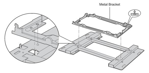
3. Attach the metal bracket to the base stands with 4 screws (B).
