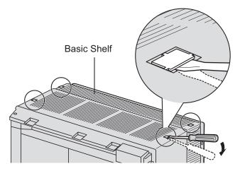
7. Lift the Basic Shelf, attach it to the metal bracket, and slide it backwards until it locks.
