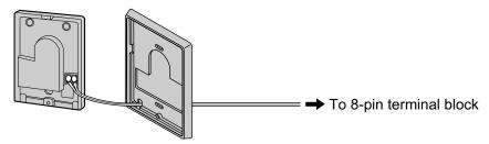
4. Re-attach the 2 halves and re-insert the screw.
