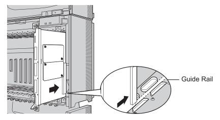
**3.** Push the release lever in the direction of the arrow so that the BUS-M card engages securely with the connector on the back board.
