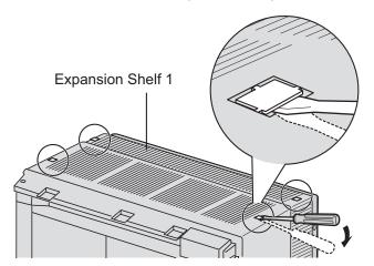
**3.** Fasten the wall brackets loosely to Expansion Shelf 1 with 4 screws (D). (This makes it easy to adjust the position of the shelves later.)
