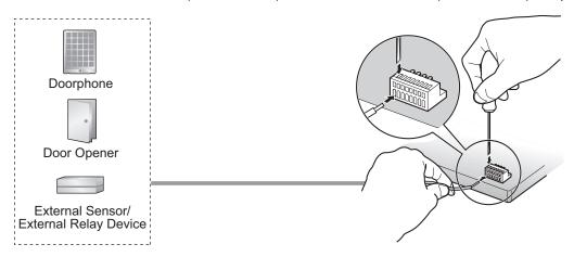
2. Attach the terminal blocks to the connectors of the DPH4/EIO4 card on the PBX.
