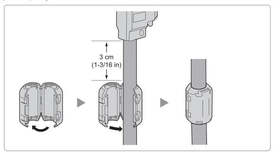
If you need to open the ferrite core, use a flathead screwdriver to unlatch the case of the ferrite core.
