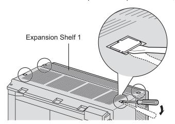
3. Lift Expansion Shelf 1, attach it to the metal bracket on the Basic Shelf, and slide it backwards until it locks.
