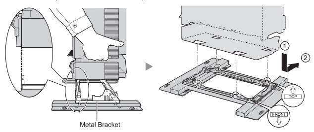
8. Secure the Basic Shelf to the metal bracket with 2 screws (B).
