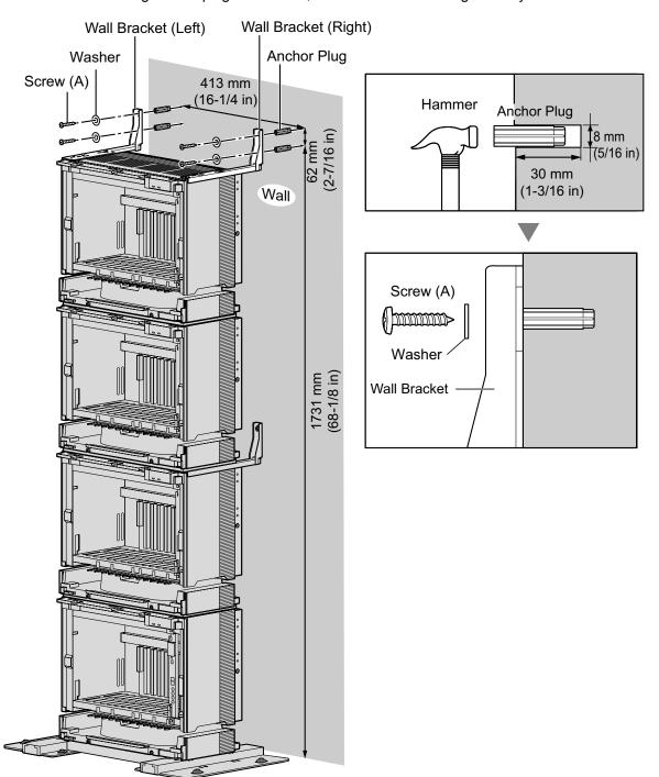
2. Check that the shelves are standing exactly vertically. If the upper shelves are leaning slightly to one side, move Expansion Shelf 3 to adjust the position. (Since the wall brackets are attached loosely to Expansion Shelf 3, it should be possible to adjust the position of the shelves.)
