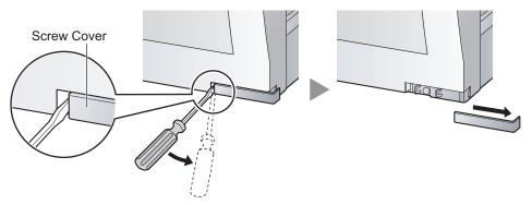
2. Turn the screw counterclockwise to loosen.
