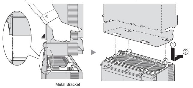
4. Secure Expansion Shelf 1 to the metal bracket with 2 screws (B).
