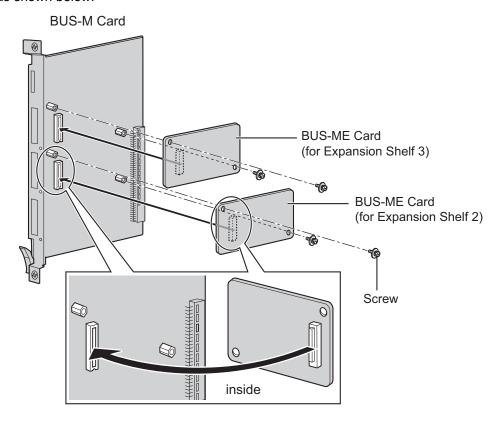
2. Insert the BUS-M card along the guide rails in the BUS-M Card Slot (the right-most slot) of the Basic Shelf.
