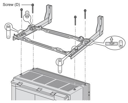
**3.** Install 4 anchor plugs in the wall, using the wall brackets as a template. Fix the wall brackets to the wall with 4 screws (A).
