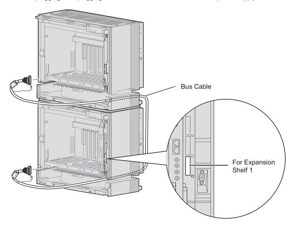
**5.** Attach the noise shield wires of the Bus Cable to the Basic Shelf and Expansion Shelf 1 with the screws of the BUS-M card.
