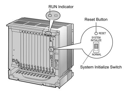
2. Plug the AC power cord into the PBX and an AC outlet, and turn on the PBX. The RUN indicator will flash.
