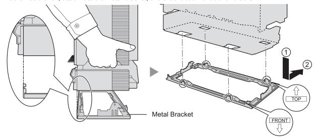
3. Secure the Basic Shelf to the metal bracket with 2 screws (B).
