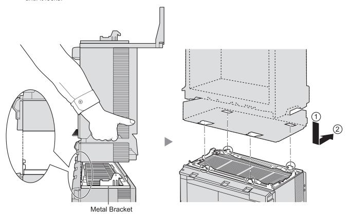
**6.** Secure Expansion Shelf 3 to the metal bracket with 2 screws (B).
