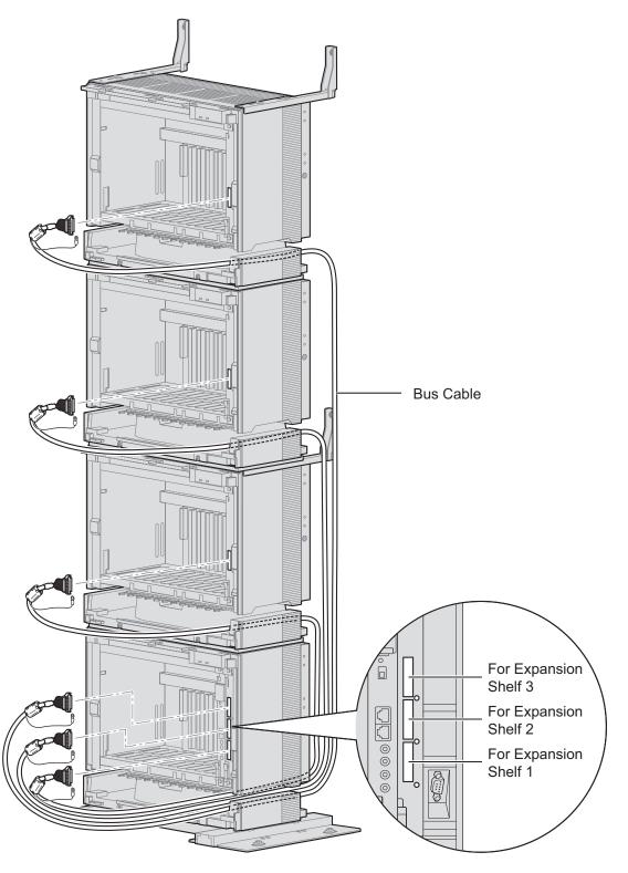
**6.** Attach the noise shield wires of each Bus Cable to the Basic Shelf and each Expansion Shelf with the screws of the BUS-M card.
