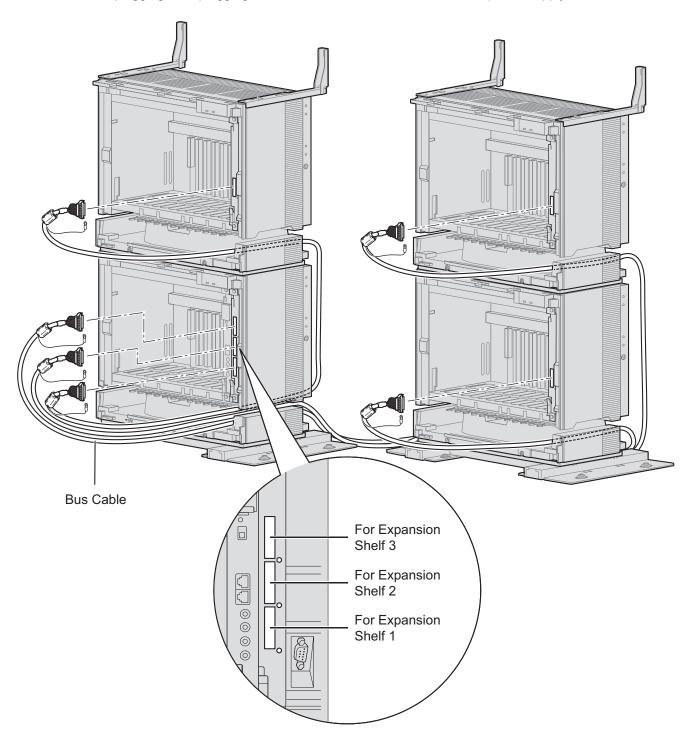
**6.** Attach the noise shield wires of each Bus Cable to the Basic Shelf and each Expansion Shelf with the screws of the BUS-M card.
