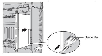
2. Push the release lever in the direction of the arrow so that the BUS-M card engages securely with the connector on the back board.
