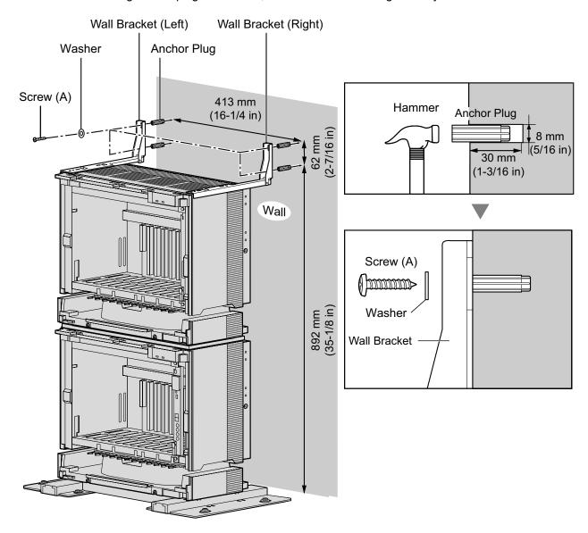
2. Check that the shelves are standing exactly vertically. If the shelves are leaning slightly to one side, move the base stands to adjust the position. (Since the base stands are attached loosely to the floor, it should be possible to adjust the position of the shelves.)
